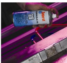
**FORMULA 14** is a non-silicone based release agent, specially developed for the mould release of thermoplastics which require post mould process treatment (painting, printing, thermo-welding, etc).
